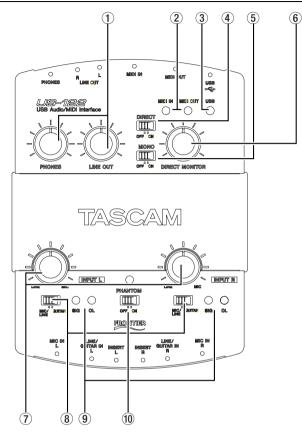
(1) **LINE OUT level control** Controls the level to the RCA outputs.
