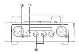
(f) MIC IN L and R Balanced XLR Inputs L and R for microphones.
