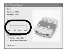
To adjust the buffer size, run the US-122 Control Panel. The *Latency* slider lets you change the buffer size from a minimum of 256 samples (128 samples on the Mac) to a maximum of 2048 samples. All audio programs that use the US-122 must quit before a new audio latency setting takes effect.
